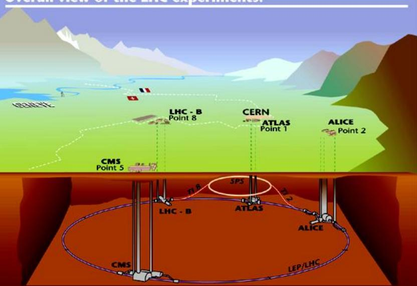
Tunnel circumference 26.7 km, tunnel diameter 3.8 m Depth : ~ 70-140 m - tunnel is inclined by ~ 1.4%
